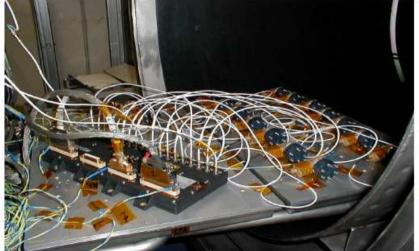
AC: 15 PMTs channels each ones with programmable HVs and gain
